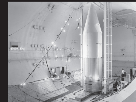
The large test chamber was used to qualify the shroud jettison system for the Orbiting Astronomical Observatory (OAO-1), a predecessor of the Hubble Telescope, in 1965. Both the Agena second-stage spacecraft and the OAO satellite were enclosed by the clam-shell shroud. The shroud consisted of three sections: the fiberglass nose, the aluminum midfaring, which separated when the Agena engines ceased, and an aft fairing which fell away with the Atlas upon separation from the upper stages. The shroud was qualified in the Space Power Chambers at altitudes of 20 miles.
