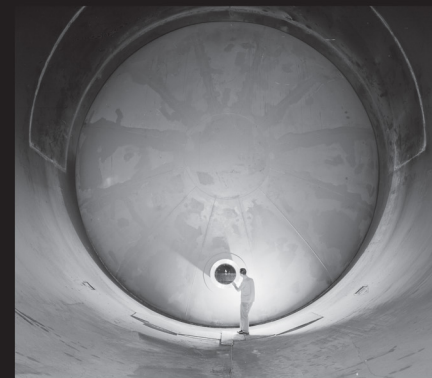
During the conversion process, three bulkheads were placed inside the tunnel to create the two test chambers. This 31-foot-diameter bulkhead was located near the southeast corner of the tunnel. A man examines a viewing portal that allowed researchers to film the tests inside the space tank on the opposite side of the barrier.
