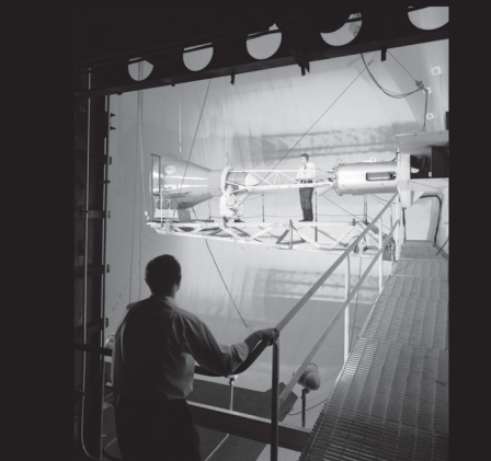
In 1959, an interior section of the AWT was gutted so that several Project Mercury tests could be conducted in altitude conditions. These included the qualification of the escape tower rocket motors, seen in this photograph. The escape rocket could jettison the Mercury capsule away from the booster in case of an emergency. Three different motors were successfully fired in the tunnel, and thrust misalignment was studied on a fourth rocket.
