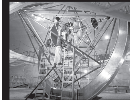
The Multiple Axis Space Test Inertial Facility, referred to as the gimbal rig or MASTIF, was initially installed in the facility to test the guidance system for Project Mercury's Big Joe capsule. It was modified afterwards to train the Mercury astronauts how to bring a tumbling spacecraft under control. An astronaut was secured in a foam couch at the center of the rig. The rig then spun along three axis at up to 30 rotations per minute. Using controls identical to actual flight equipment, they operated small nitrogen jets on the cages to slow and gain control of the rig.
