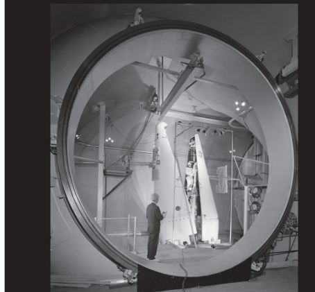
After an error during the separation of the stages on the Atlas/Centaur-3 flight, NASA Lewis researchers conducted a series of shroud jettison tests in the Space Power Chambers' vacuum chamber. A new shroud was designed and the original test procedure was modified. The separation on the December 11, 1964, Atlas/Centaur-4 launch was flawless. In 1965, the SPC was used to qualify a modified shroud for the Atlas/Centaur-6 mission, which would be the first successful placement of the Surveyor model into an elliptical Earth orbit.
