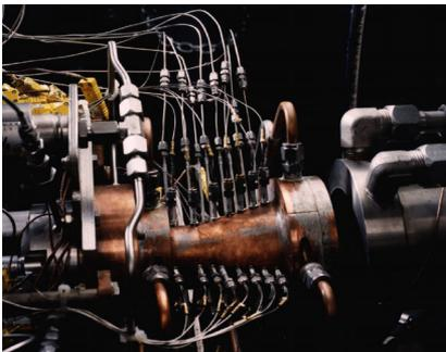
**RCL-11 Instrumented Chamber for 25-lbf Nozzle Study**
