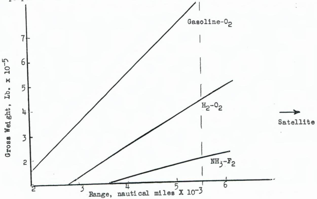
This figure also shows that as range increases the need for high-energy propellants increase.
