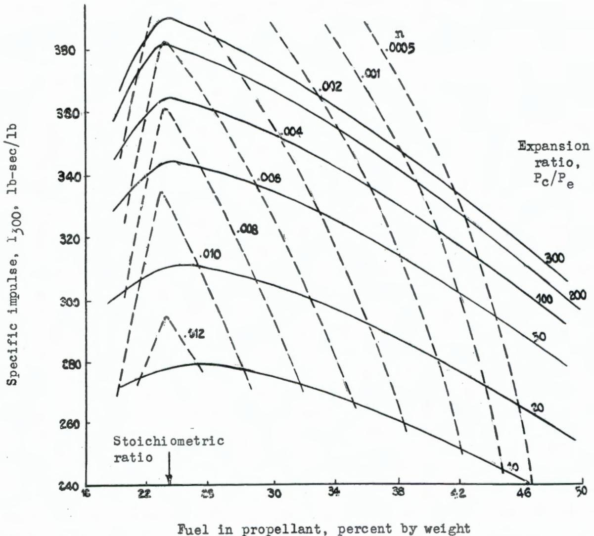
To obtain the specific impulse at any pressure use the equation
