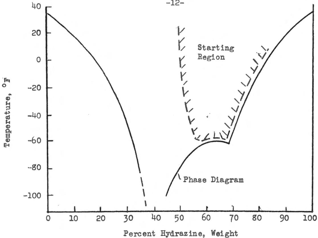
Starting fuels which are miscible with gasoline do not behave in the same way, and this suggests that a separate ignitor chamber directing a flame into the combustion chamber would be more reliable and would permit attainment of satisfactory starts at  $-76^{\circ}\text{F}$  or below.
