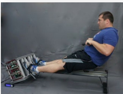
Breadboard ROCKY being used in resistive mode as a rowing machine (slide not necessary in 0-g)
