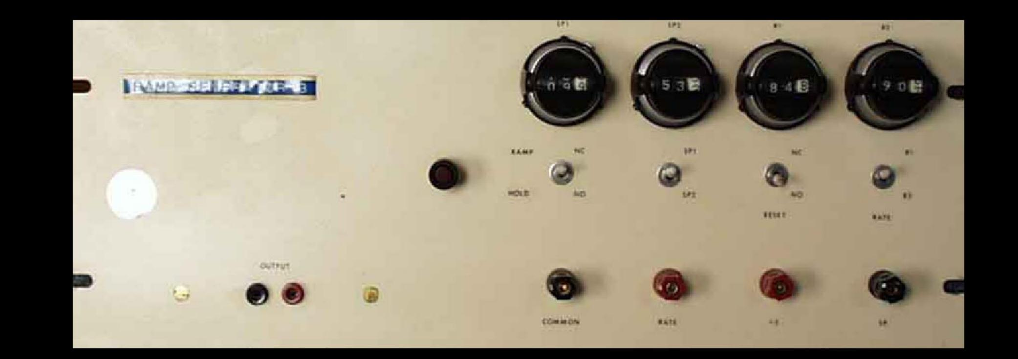
This panel and electronic equipment controlled the speed at which the valves were opened to allow the fuel and oxidizers into the test cell.
