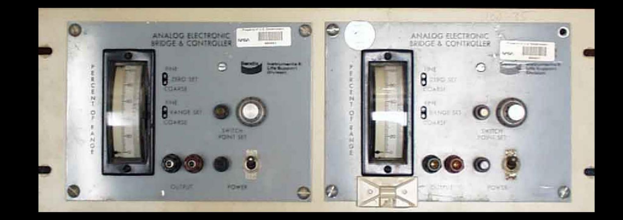
This is a ramp generator panel. According to former RETF Engineer Doug Bewley, "These ramp-generators were used to provide reference electrical signals to the controllers who then positioned the valves that provided the liquid oxygen and liquid hydrogen to the rocket engine being tested."
