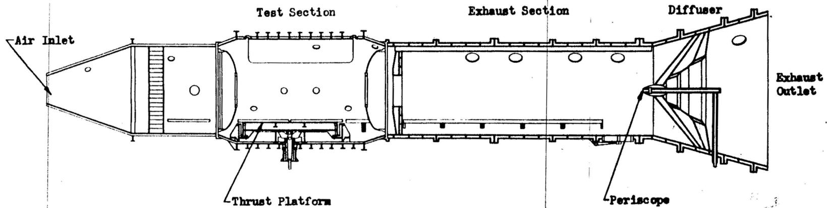
Fig.45 Diagram of Propulsion Sciences Laboratory Altitude Test Chamber
