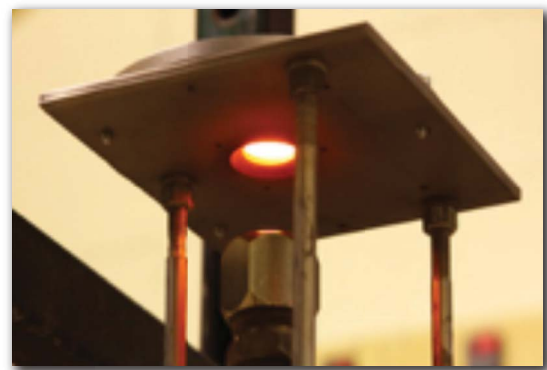
Button coupon under thermal gradient conditions can simulate thermal stresses and provide in situ thermal conductivity measurements.
