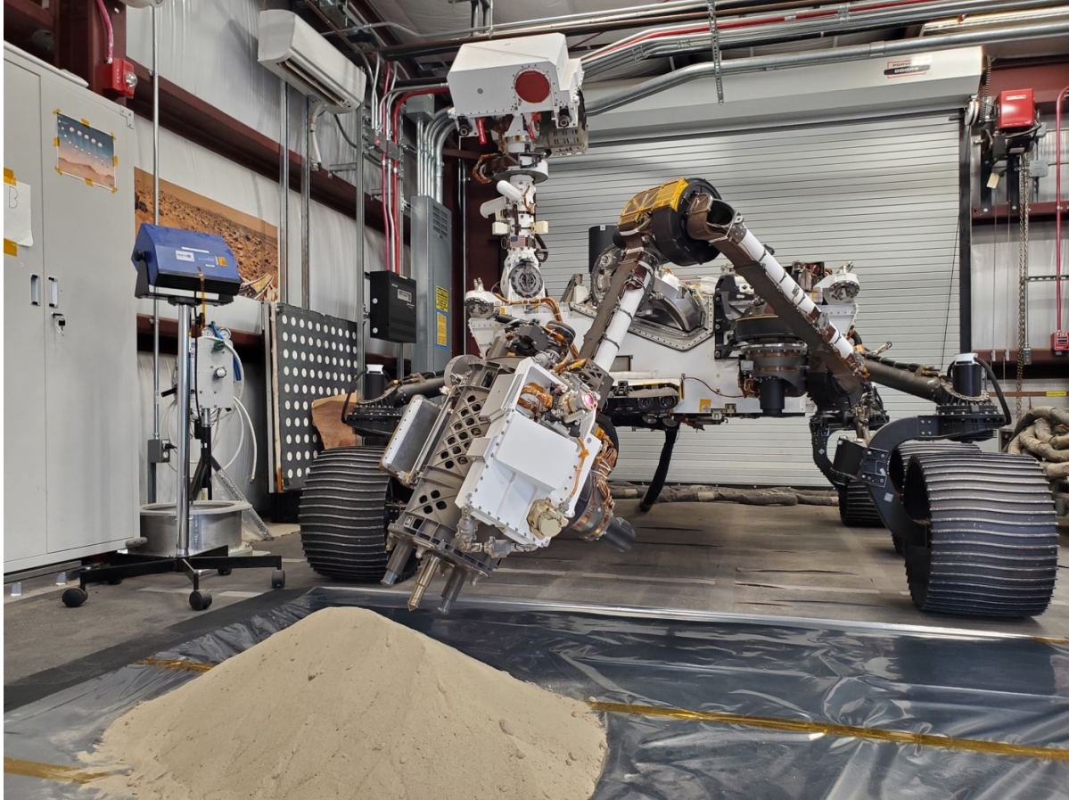
Figure 3: Picture of the full-scale Earth replica of the Perseverance robot. It has wheels for mobility, a robotic arm for positioning science instruments and tools close to the surface. It is shown here using its robotic arm to position the regolith bit for sampling. It is comparable in scale to the Curiosity rover show in Figure 1(b) [3].
