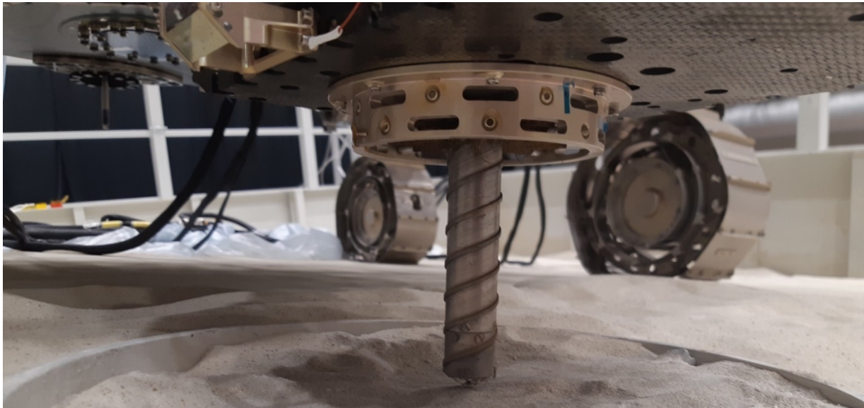
Figure 9: Image of the Ground Test Model of the European Space Agency Rosalind Franklin rover drill that would penetrate 2 meters beneath the surface to retrieve samples and deliver them to instruments [38].
