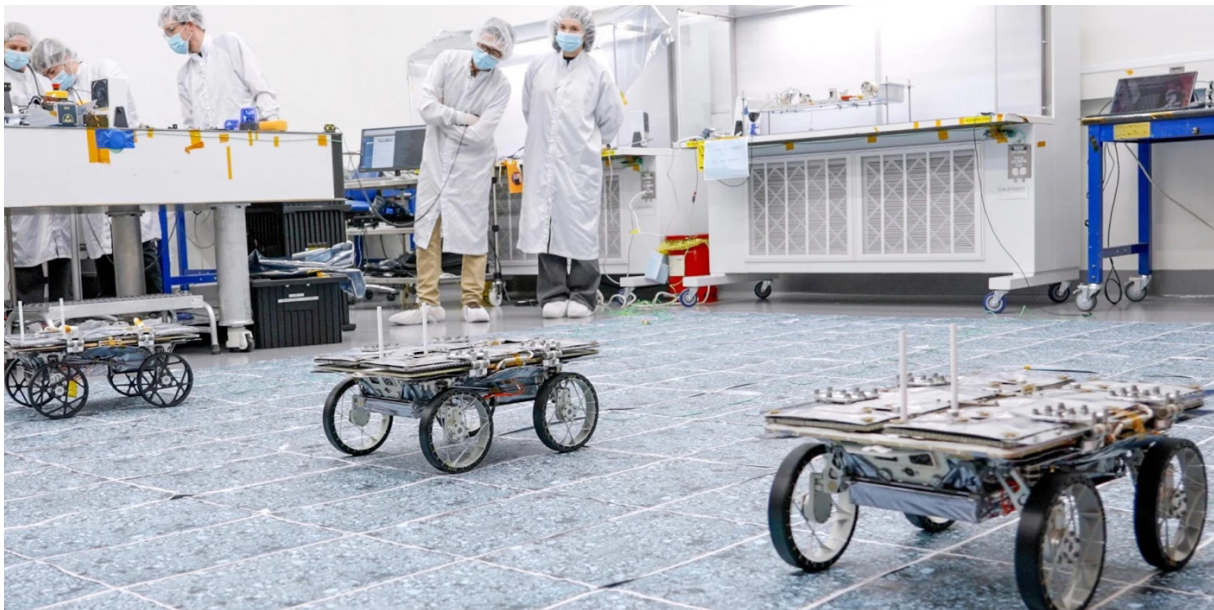
Figure 8: Image of the three CADRE rovers (~9kg each) designed for a CLPS lunar technology demonstration [3].
