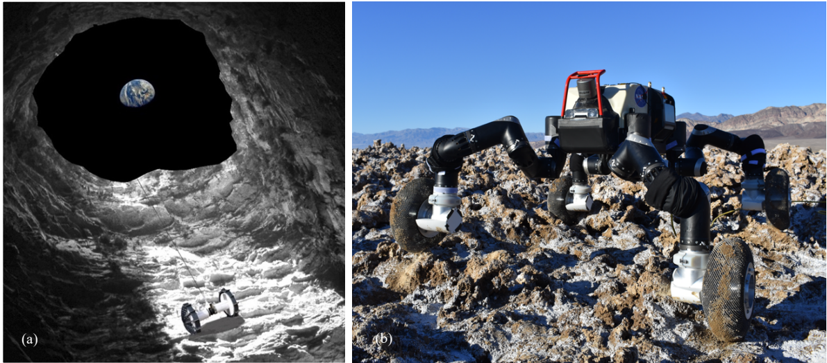
Figure 16: (a) Illustration of the Moondiver Discovery concept to explore extreme terrain on the Moon. (b) Image of the RoboSimian robot in its actively articulated wheel-on-limb rover form to traverse unstructured planetary analogue terrain. It was originally developed as a mobile manipulation platform for the DARPA Robotics Challenge [3].
