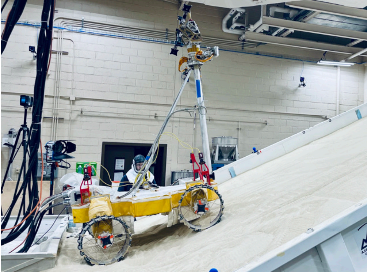
Figure 7: A test model of VIPER illustrates chassis body leveling via active suspension adjustments. The rover is 1.7x1.7x2.5m and weighs 490kg [28].
