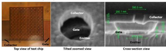
**Q3/Y2 – Y3:** Si NVCTs with on-chip components were fabricated on 6" wafers. Devices characterized. Circuit demo work is in progress.
