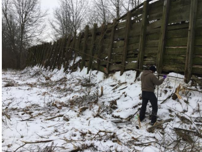
Figure 2-7. Soil Sample Collection along Decaying Blast Wall of Firing Range 3
