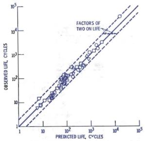
Predicting fatigue life by an analytical technique called Strainrange Partitioning
