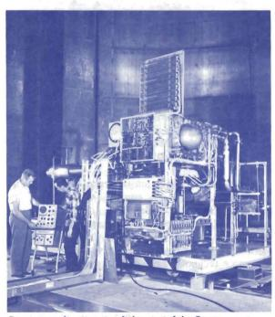
Brayton cycle generator being tested in Space Power Facility
