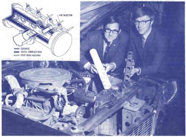
Experimental thermal reactor for automobile pollution control
