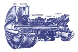
Typical high bypass ratio engine
