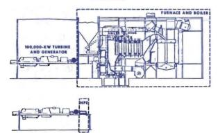
Size comparison of coal fired steam plant for electric power generation with one using rocket type combustor
