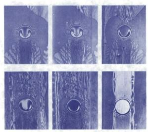
Photomicrograph of progressive lubricant starvation of bearing
