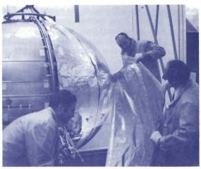
Insulating a liquid hydrogen tank
