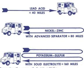
Increasing the range of electric vehicles (1000 lbs of batteries)
