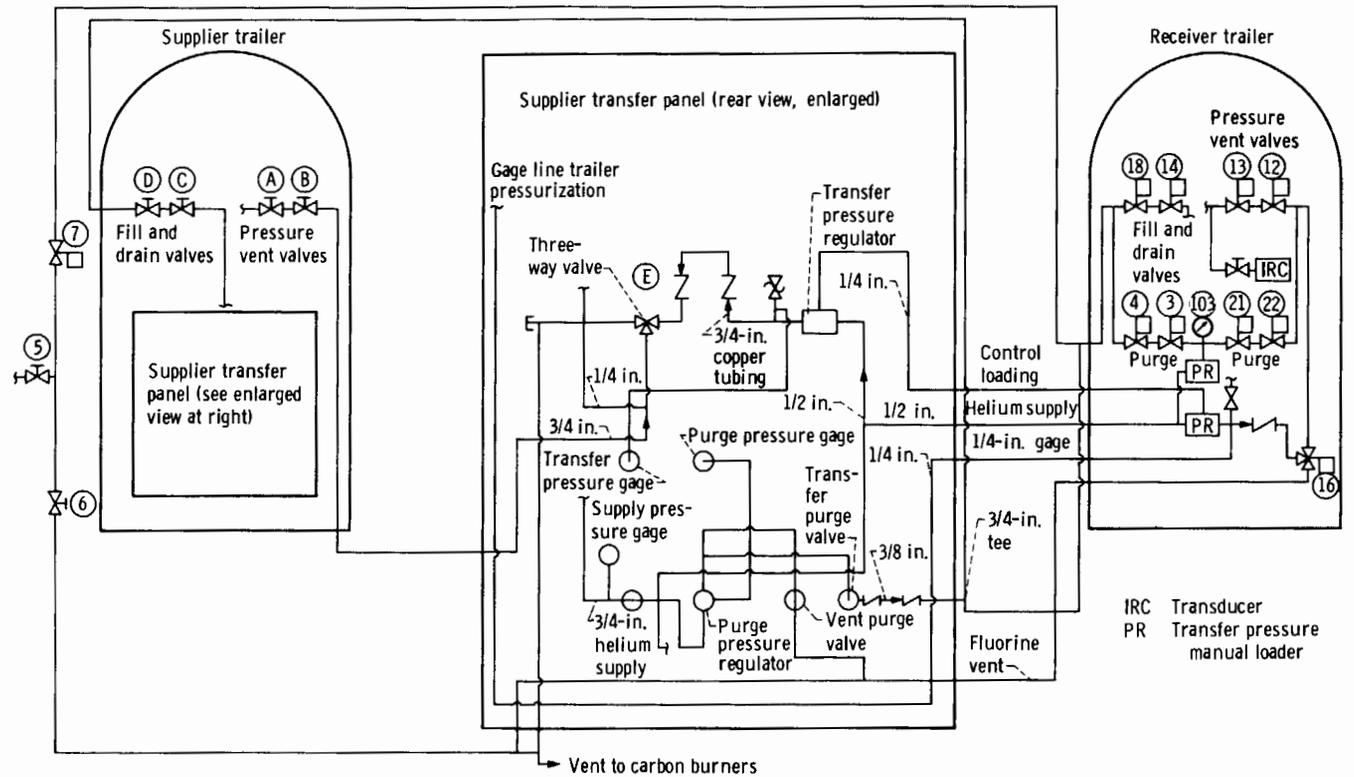
FIGURE 8-1.—Liquid-fluorine transfer valves and gages.
