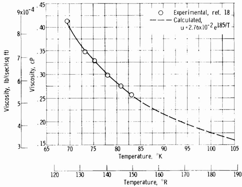
FIGURE 2-8.—Viscosity of liquid fluorine.
