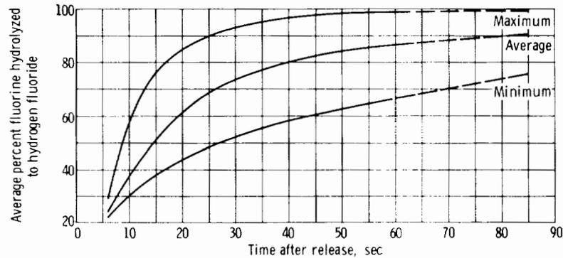
FIGURE 5-4.—Reaction of fluorine with atmospheric moisture to form hydrogen fluoride (data from ref. 3).
