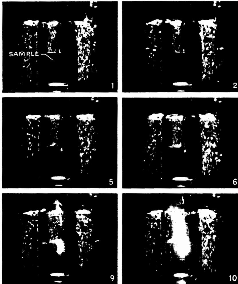
FIGURE 3-16.—Typical slow-burning surface reaction of neoprene
