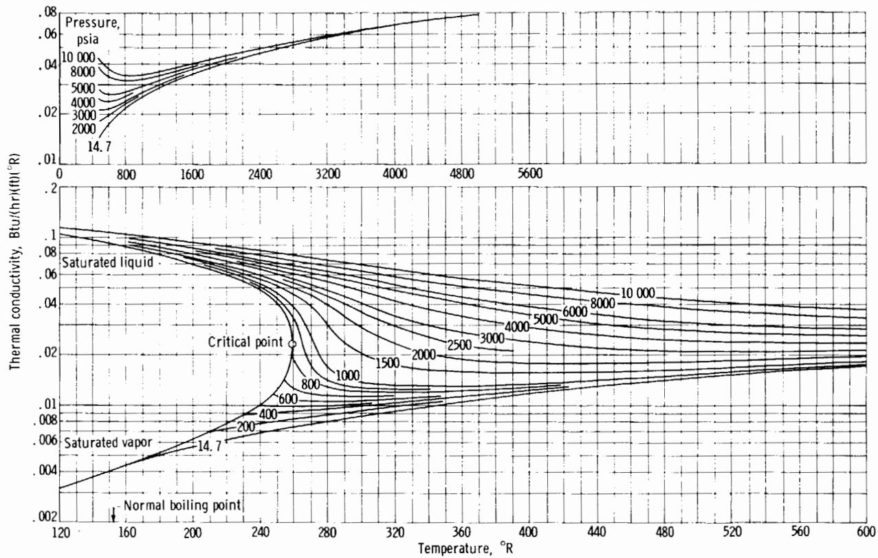
FIGURE 2-10.—Thermal conductivity of fluorine (ref. 23).
