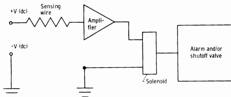
FIGURE 5-6.—Schematic drawing of burglar-alarm system.
