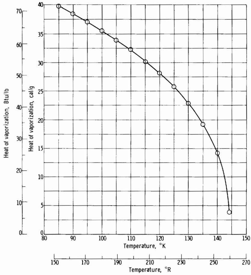
FIGURE 2-4.—Heats of vaporization of fluorine (ref. 13).
