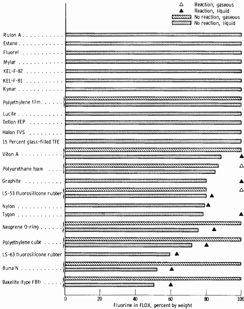
FIGURE 3-15.—Static compatibility test results for solid nonmetals in FLOX. Liquid FLOX temperature,  $-320^{\circ}$  F; gaseous FLOX temperature,  $20^{\circ}$  to  $40^{\circ}$  F; pressure, atmospheric (ref. 24). (These results should not be used as a guide in selecting materials to withstand dynamic conditions or pressures greater than atmospheric.)
