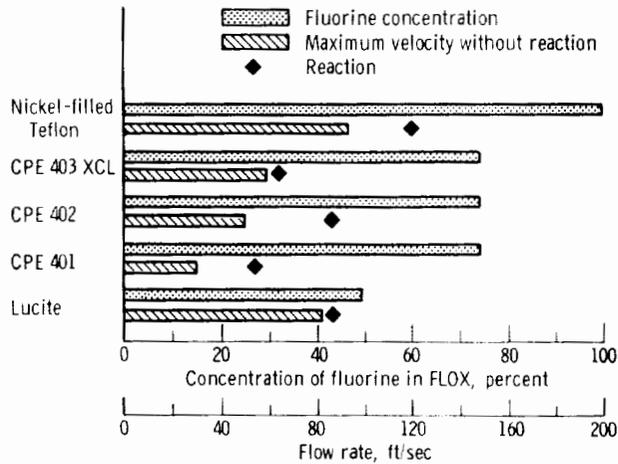
FIGURE 3-20.—Dynamic liquid FLOX compatibility tests (single data points, ref. 24). Pressure range, 100 to 400 pounds per square inch gage; temperature,  $-320^{\circ}\text{F}$ ; specimen configuration, 0.25-inch orifices.
