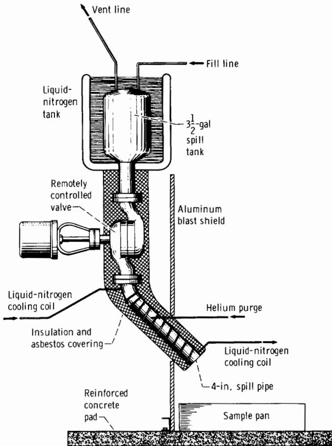
FIGURE 3-25.—Apparatus used for FLOX spill tests (ref. 25).
