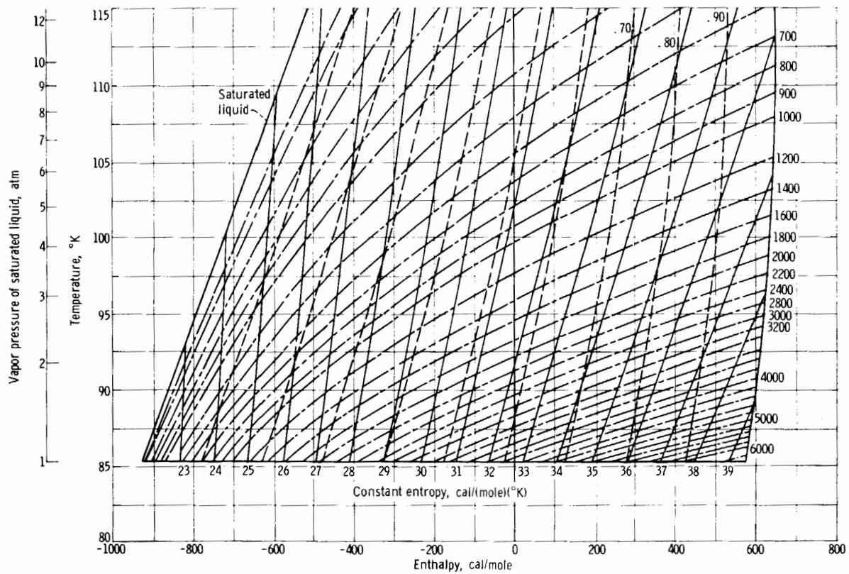
FIGURE 2-5.—Temperature-enthalpy diagram for fluorine (ref. 13).
