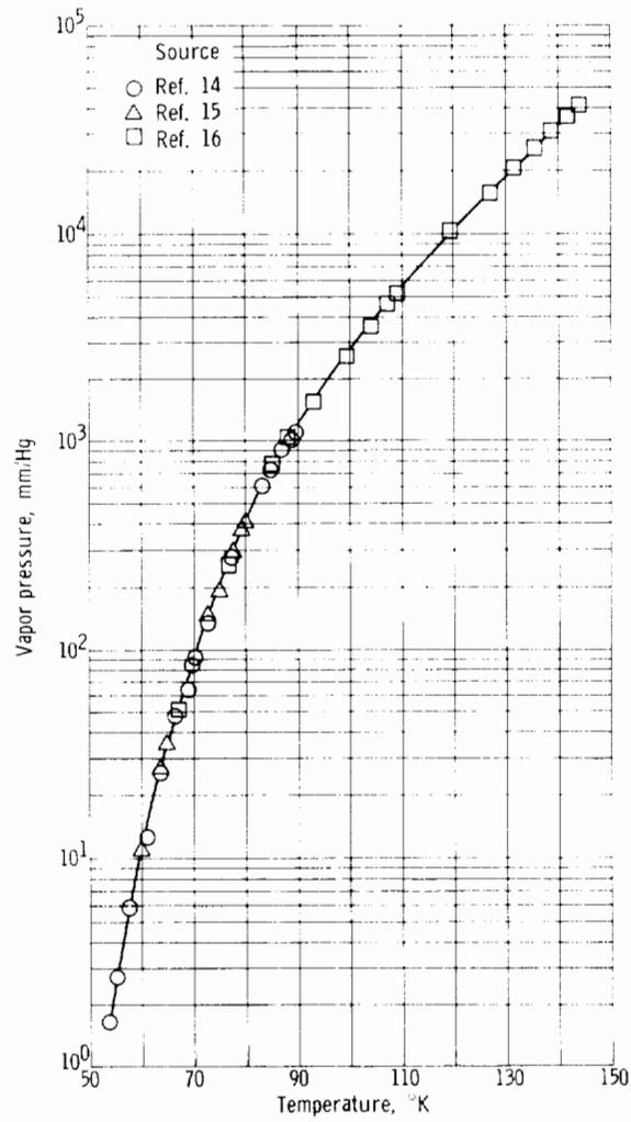
FIGURE 2-2.—Vapor pressure of liquid fluorine.
