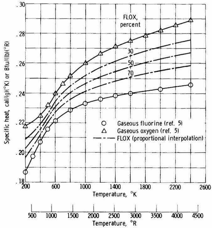
FIGURE 2-20.—Specific heat of gaseous-fluorine-gaseous-oxygen mixtures at 1 atmosphere.
