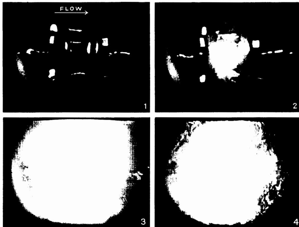
FIGURE 3-21.—Dynamic FLOX compatibility test of Lucite specimen. Film speed, 24 frames per second; time interval between frames, 1 and 2, and 3 and 4, 9 seconds (ref. 24).
