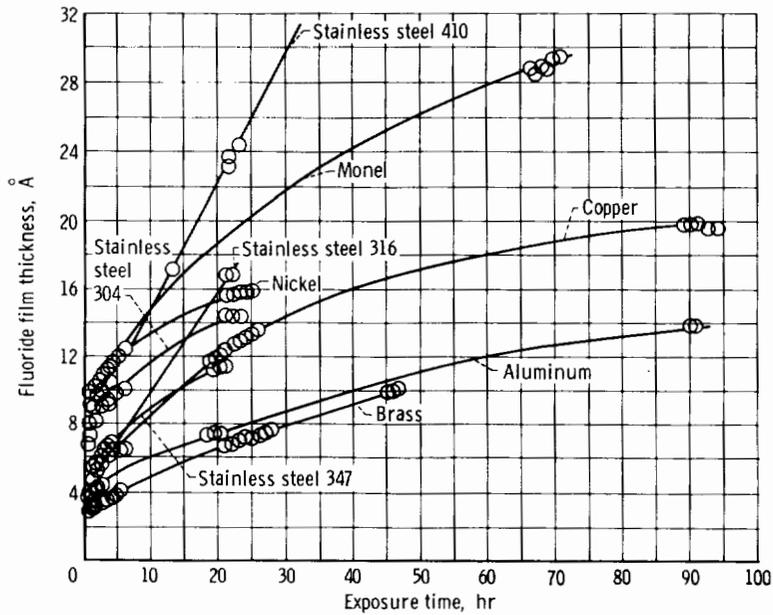
FIGURE 3-10.—Variation of film thickness on metal powders at 86° F with time of exposure to gaseous fluorine for total run (ref. 11).
