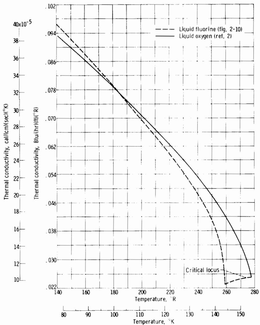
FIGURE 2-17.—Thermal conductivity of liquid fluorine and liquid oxygen.
