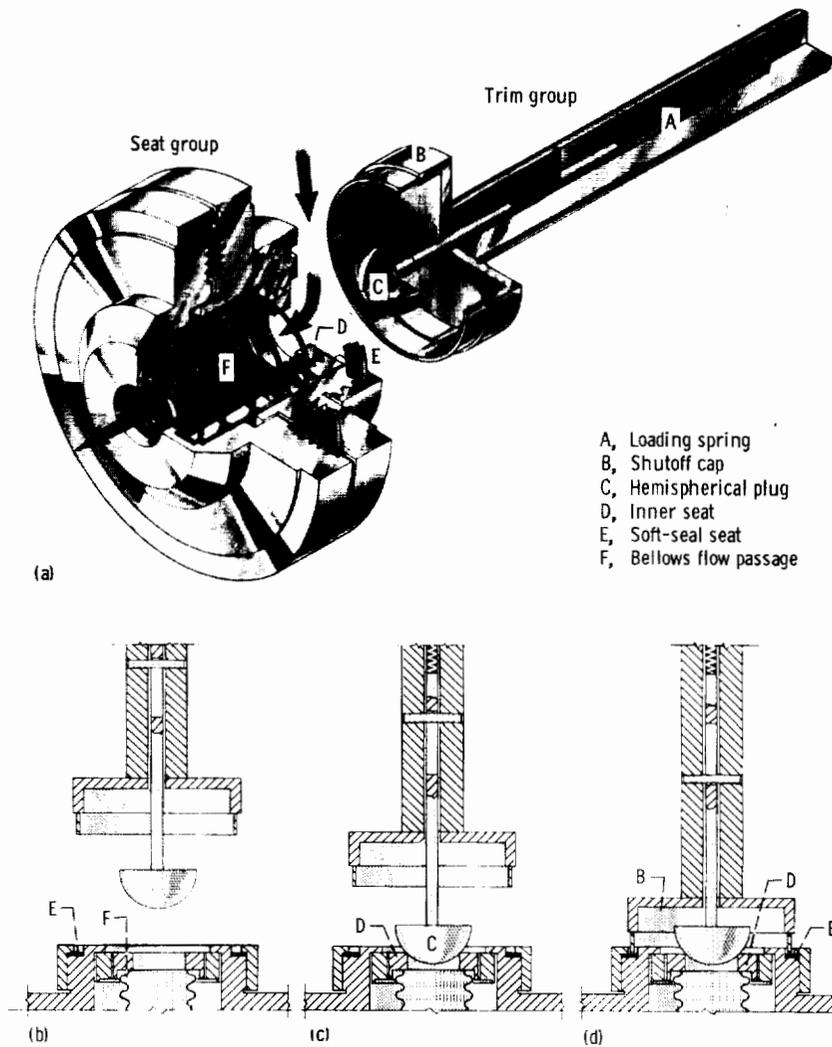
FIGURE 4-8.—Soft-seal valve developed at Lewis.
