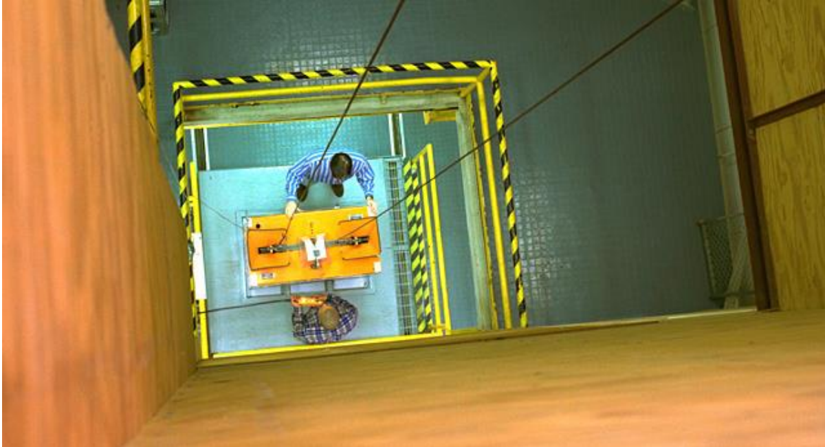
View within the 2.2 Second Drop Tower as technicians prepare for a drop test.
