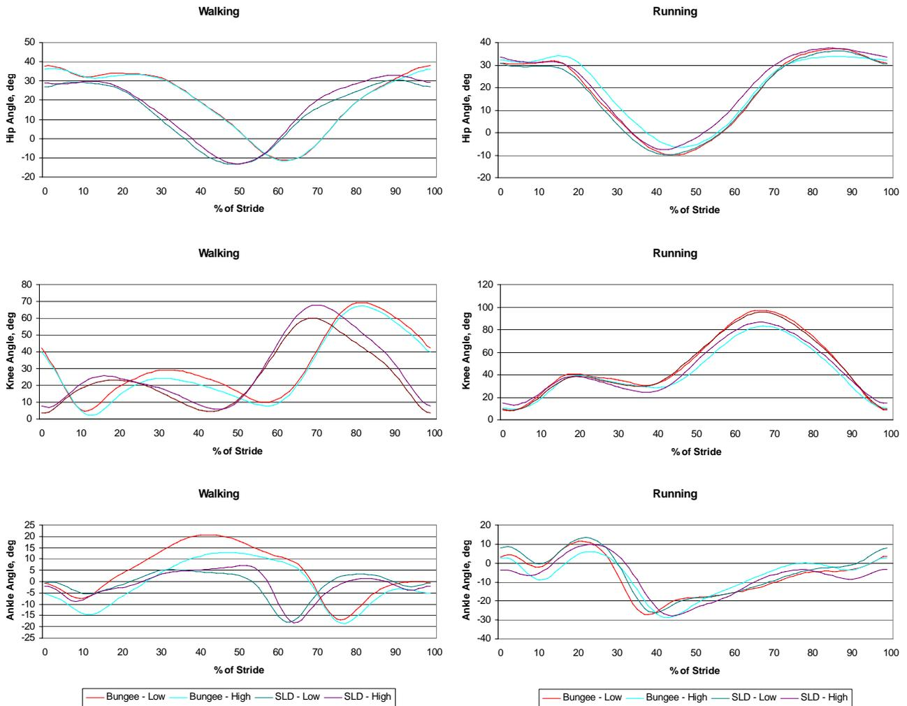
Figure 6: Joint ensemble average trajectories for a single stride for a single subject during walking and running on the eZLS while loaded with bungees and LM-SLD.
