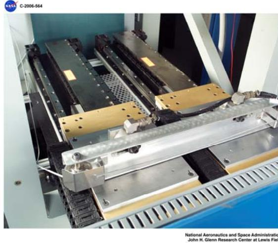
**Figure 4: Linear motor subject loading device incorporated into the eZLS.**
