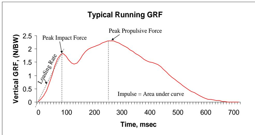
Figure 5: Typical running ground reaction force and dependent variables.
