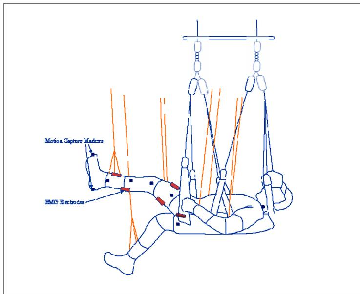
**Figure 3: Typical subject setup on the eZLS, including motion capture marker and EMG electrode placement.**
