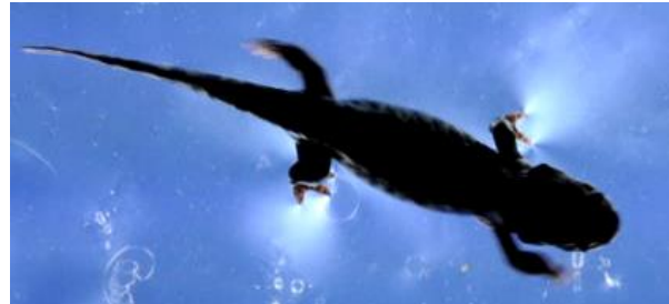
Figure 1 – A tiger salamander walking terrestrially on photoelastic gel. The bright areas at the left forefoot and right hindfoot show force application.
