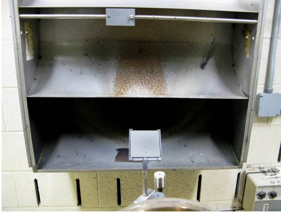
Figure 10.—Same set up as that in Figure 9 with photo taken along centerline of burner. Note lower 3- by 3-in. superalloy plate positioned to be impinged upon by flame. Upper 1.5-by 3-in. rectangular sample mounted to the duct is polymeric.
