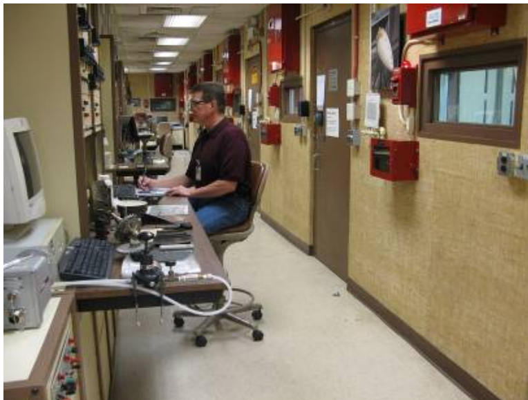
Figure 4.—Burner rig facility control room. The burner rig is housed in test cell behind the operator as he sits at the control PC.
