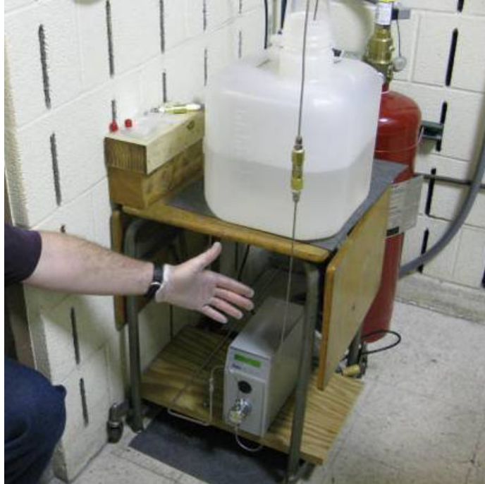
Figure 2.—Current means used to add alternate fuel (e.g., Fischer–Tropsch) to the primary jet fuel is with a positive displacement, reciprocating piston pump.
