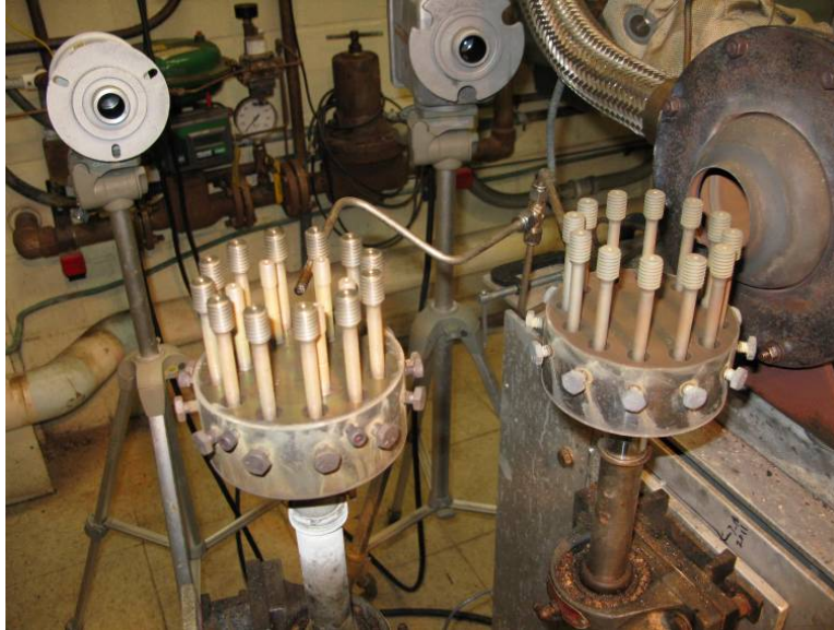
Figure 11.—Carousels holding superalloy tensile specimens. Samples were subjected to corrosive species to determine the effect on mechanical properties.
