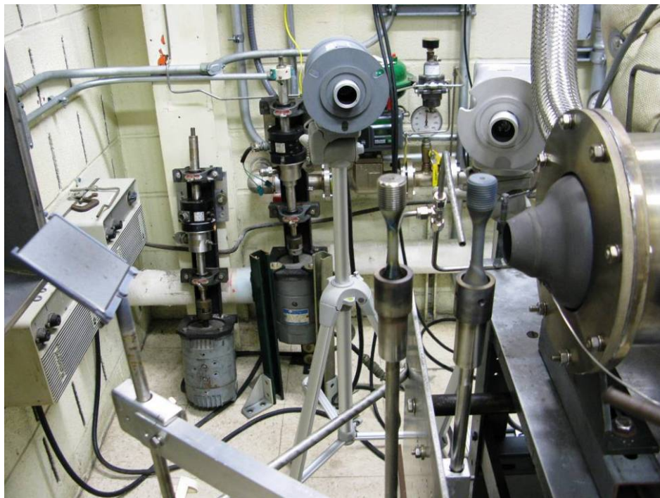
Figure 9.—Durability testing of a TBC-coated 3- by 3-in. superalloy plate (at left in photo), carried out at the same time as two fixed superalloy “dog bone” specimens. Exhaust nozzle diameter is 1.9 cm (0.75-in.).
