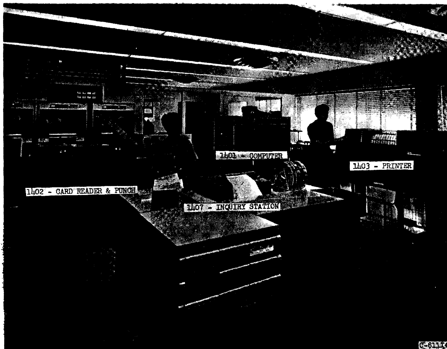
Figure 49. - 1401 system showing 1401 computer, 1402 card reader and punch, and 1403 printer.
