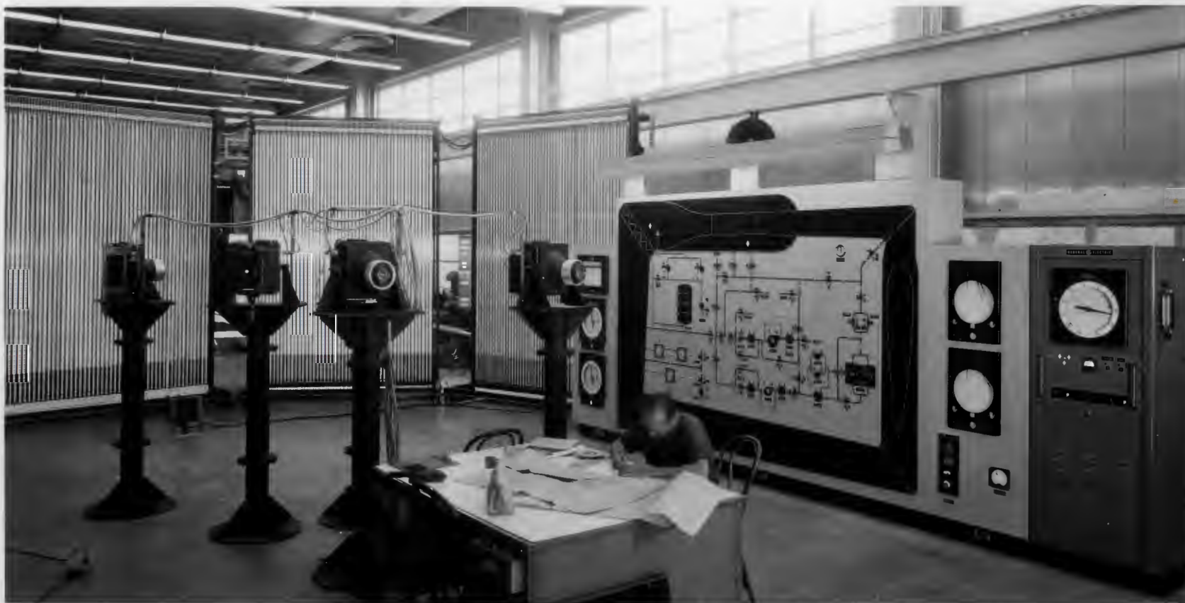
(b) Control and Data Center of the 8-Foot Transonic Pressure Tunnel
