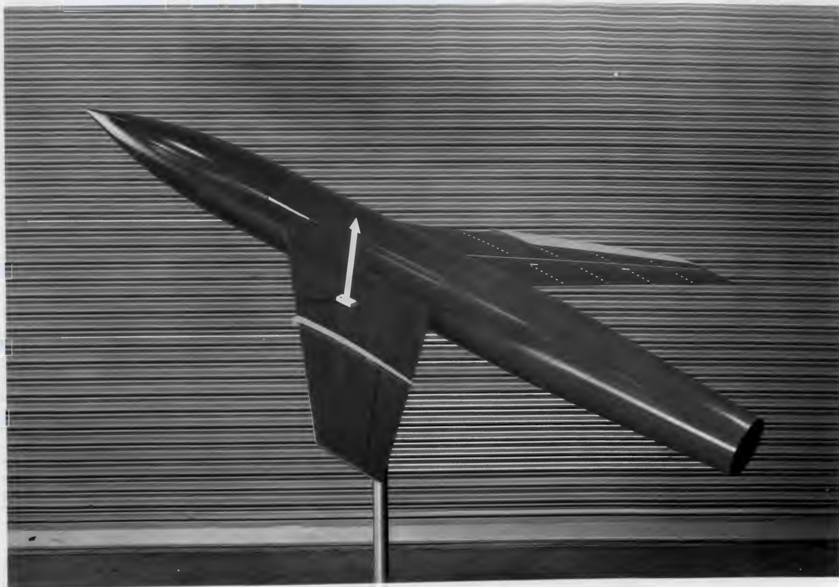
Mock-Up of a 16-Foot Transonic Tunnel Model
