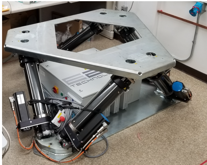
Figure 2 E2M Technologies six DOF Stewart Platform representing spacecraft lander.
